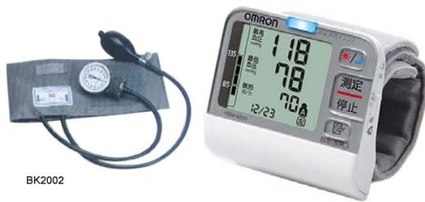
Figure 34 – Although neither of these sphygmomanometers use actual mercury, they both measure blood pressure in the unit millimeters of mercury (mm Hg.)
