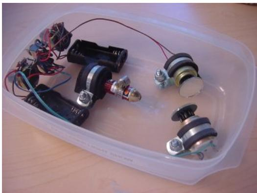
You can add potentiometers for a quick motor control as shown below and DPDT switches with a "center off" position to reverse the motor direction.
